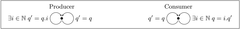
Fig. 1. Asynchronous producer-consumer protocol; q \in \mathbb{N}^* denotes the content of the shared FIFO-buffer before, q' after a transition
